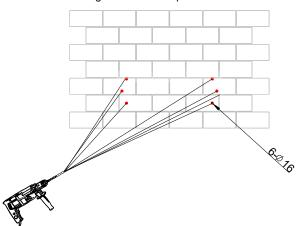
Figure 4.20. Drilling holes
