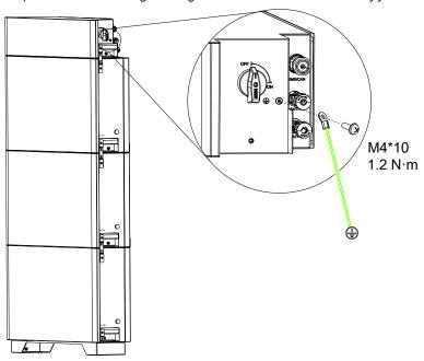
Figure 5.25. Connecting the grounding cable
