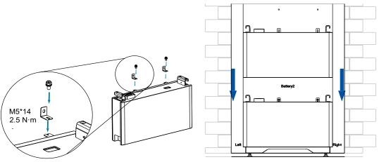
Figure 4.11. Installing the second battery
