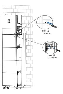
Figure 4.18. Installing the inverter
