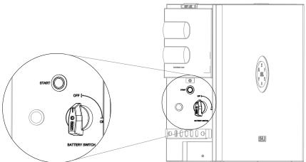
Figure 6.1. Switches on the left side of the inverter
