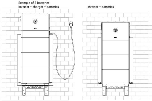
Figure 4.35. Completion view of a single stack
