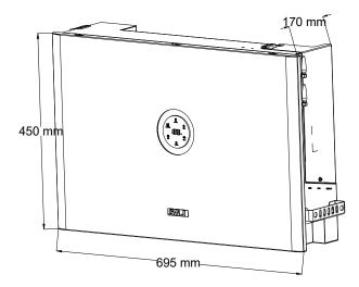
Figure 2.1. Inverter dimension
