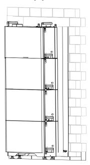
Figure 4.13. Installing the third battery
