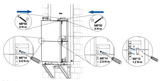
Figure 4.28. Securing the batteries
