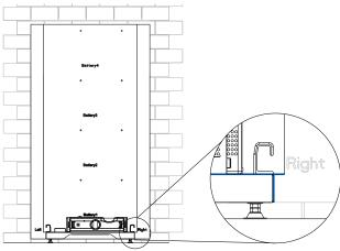
Figure 4.7. Aligning the cardboard with the battery base
