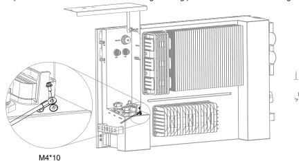
Figure 5.4. Connecting the additional grounding cable
