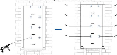
Figure 4.23. Drilling holes
