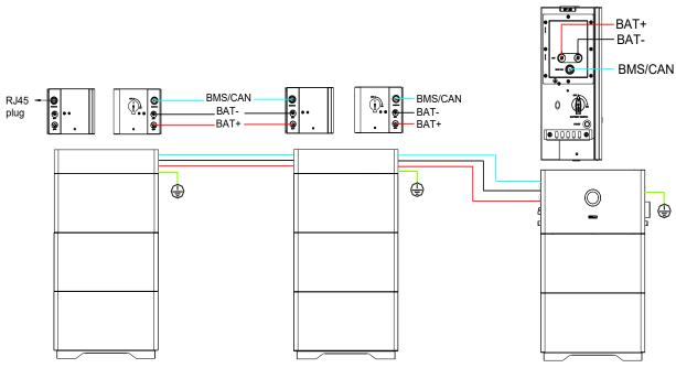
Figure 5.23. Connection of two battery stacks to inverter
