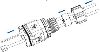
Figure 5.18. Inserting the cables through the connector
