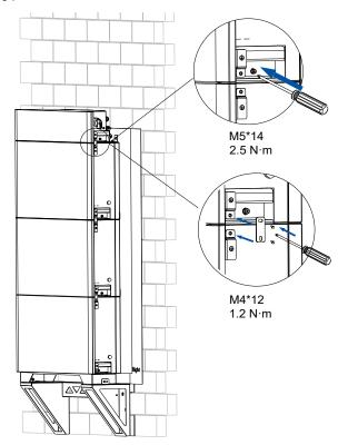
Figure 4.36. Installing a battery junction box
