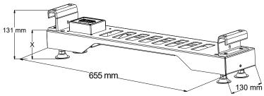
Figure 2.2. Dimension of the battery base
