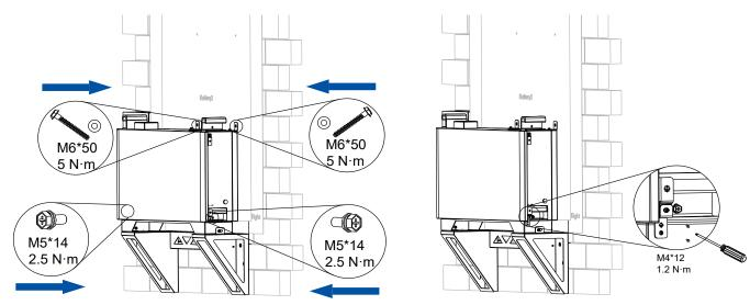
Figure 4.26. Securing the battery to the wall
