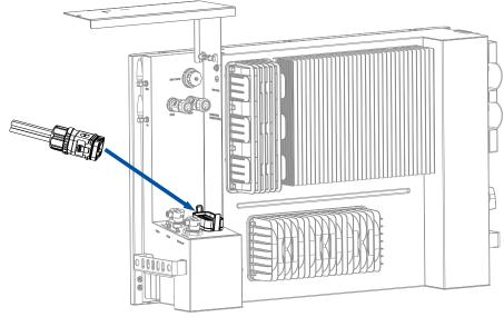
Step 6. Connect the assembled communication terminal connector to the COMM port on the inverter.
