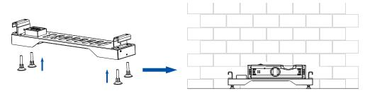
Figure 4.6. (Optional) Adjusting the battery base horizontally
