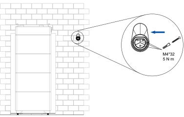
Figure 4.15. Installing the charger cable holster
