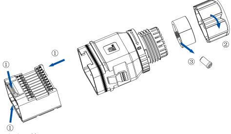
Figure 5.15. Disassembling the 24-pin communication cable connector
