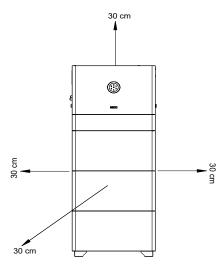
Figure 4.4. Installation clearance
