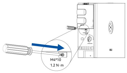
Figure 5.33. Securing the screw
