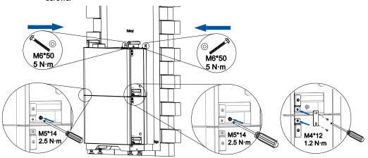
Figure 4.12. Securing the batteries
