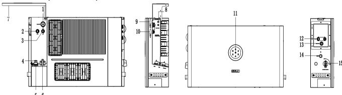
Figure 2.7. Ports, switches, and LED on the AS3 inverter
