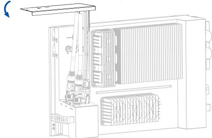
Figure 5.21. Closing the AC-side cover
