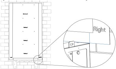
Figure 4.22. Aligning the cardboard with the bracket
