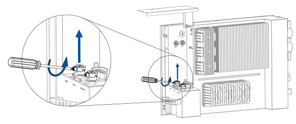
Figure 5.12. Removing the dustproof cover
