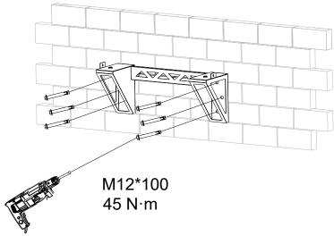
Figure 4.21. Installing the mounting bracket
