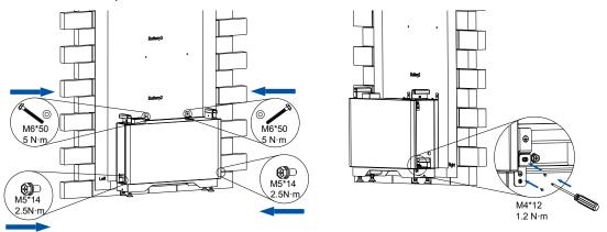
Figure 4.10. Securing the battery to the wall
