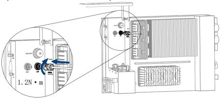
Figure 5.8. Connecting the LAN cable
