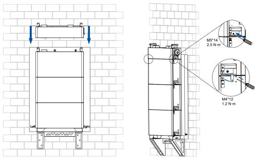
Figure 4.30. Installing the charger
