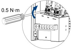
Figure 5.14. Securing the grid and backup load connectors
