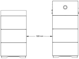
Figure 4.37. Completion view of two battery stacks
