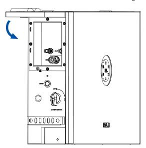
Figure 5.32. Closing the DC-side cover
