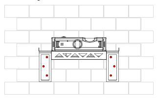
Figure 4.19. Marking the hole positions
