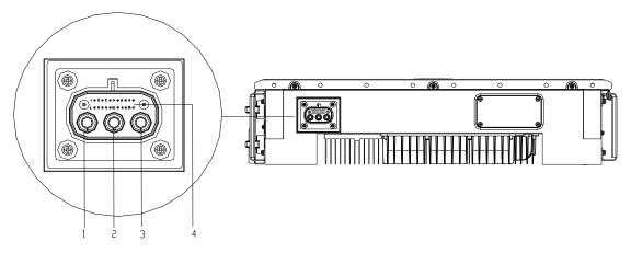
Figure 2.8. Ports of the blind-mate connector on the inverter
