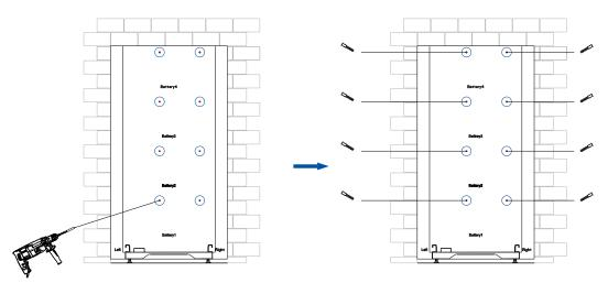
Figure 4.8. Marking and drilling holes on the wall
