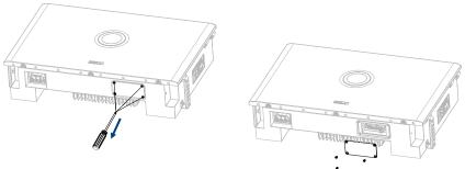
Figure 4.17. Removing the port cover
