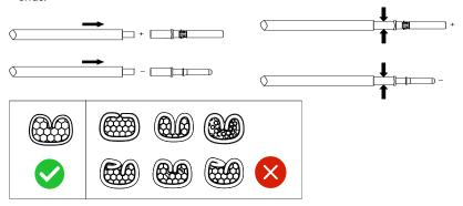
Figure 5.27. Inserting to the sleeves
