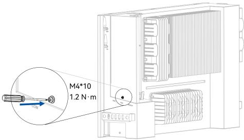
Figure 5.22. Securing the screw
