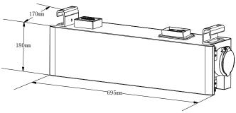
Figure 2.6. Dimension of the CU2 charger B
