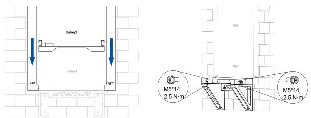
Figure 4.24. Installing the battery base
