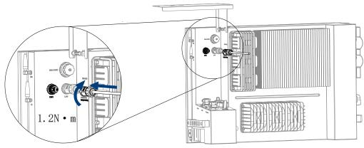
Figure 5.10. Connecting the EMS cable
