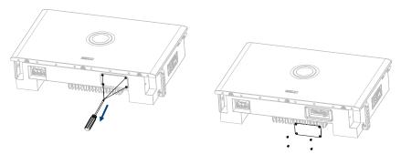
Figure 4.33. Removing the port cover
