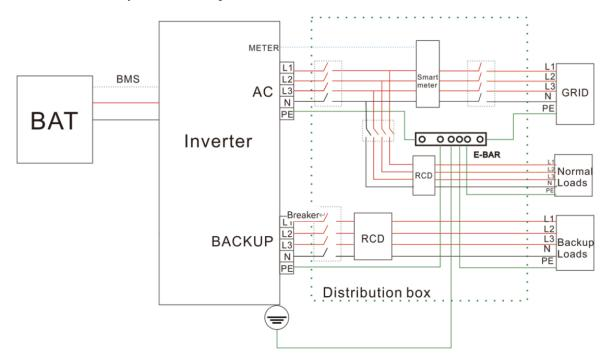
Figure 5.34. System connection
