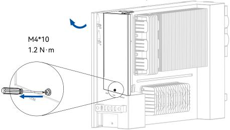
Figure 5.1. Opening the AC-side cover
