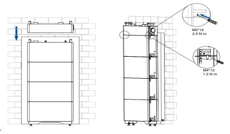
Figure 4.14. Installing the charger
