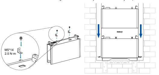
Figure 4.27. Installing the second battery
