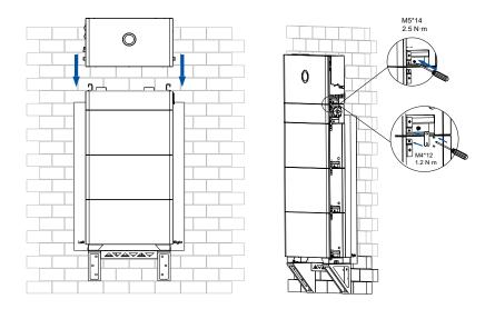
Figure 4.34. Installing the inverter
