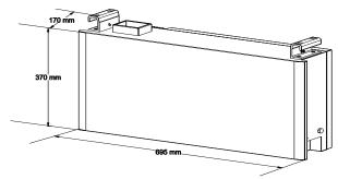
Figure 2.3. Dimension of the battery pack
