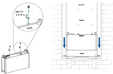
Figure 4.25. Installing the first battery
