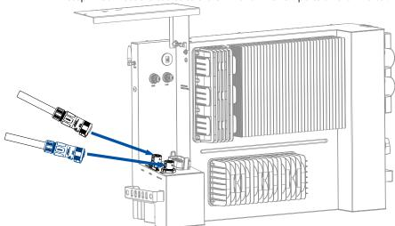
Figure 5.13. Connecting the grid and backup load cables
