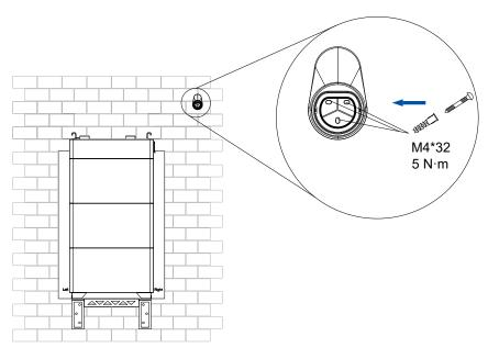
Figure 4.31. Installing the charger cable holster
