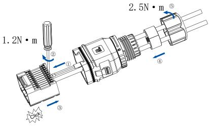
Figure 5.19. Assembling the connector
