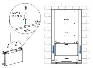
Figure 4.9. Installing the first battery
