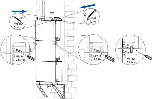
Figure 4.29. Installing the third and fourth battery
