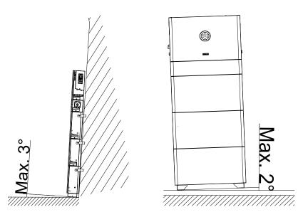
Figure 4.3. Installation angle
