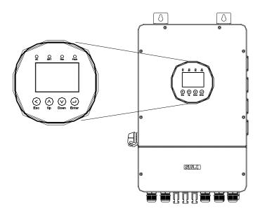
Figure 2.5 LCD indicators and buttons
