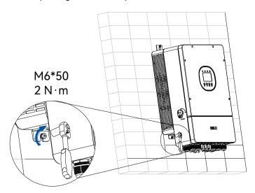
Figure 4.10. Secure the inverter
