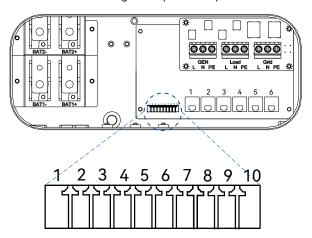
Figure 5.16. Communication ports
