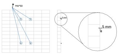
Figure 4.8. Install the mounting bracket onto the wall
