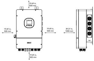
Figure 4.5. Installation clearance
