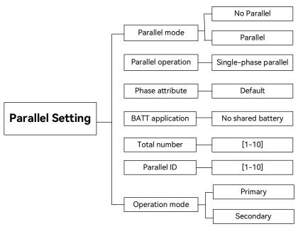
By default, the inverter configured with **Parallel ID 1** will work as the primary device (in the **Primary** operation mode). If you assign **Primary** mode to another inverter (e.g., **Parallel ID 2**), the device configured with **Parallel ID 1** will switch to **Secondary mode**.
