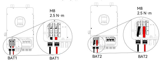
Figure 5.5. Connect the battery cables
