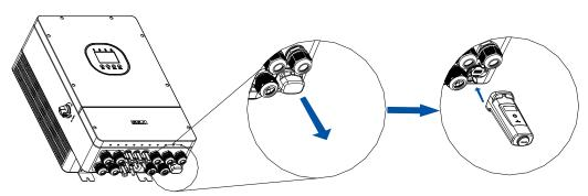
Figure 5.7. Installing the communication module
