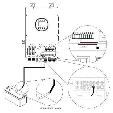
Figure 5.8. Connecting the battery temperature sensor
