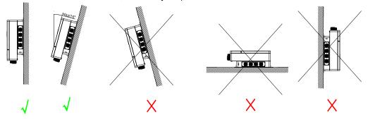
Figure 4.4. Installation position
