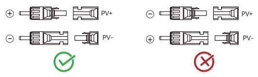
Figure 5.23. Connecting the connectors into terminals
