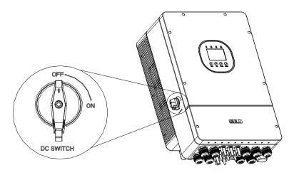
Figure 5.22. Turning OFF the DC switch
