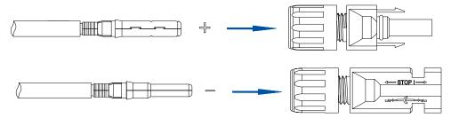
Figure 5.20. Inserting the assembled cables into connectors
