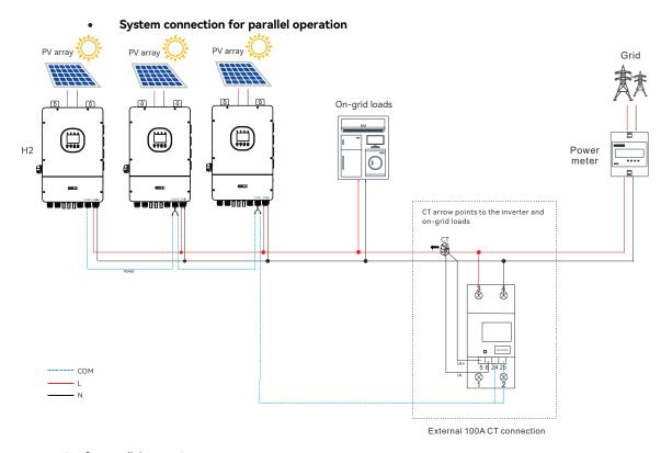
Figure 5.12. System connection for parallel operation
