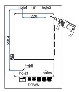
Figure 4.7. Drill four holes on the wall
