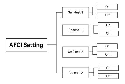
With the Arc-fault circuit-interrupter (AFCI) protection, when there is an arc signal on the DC side due to aging of the cable or loose contact, the inverters can quickly detect it and cut off the power to prevent fire and ensure the PV system safety.
