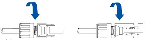
Figure 5.21. Tightening the lock screws on connectors
