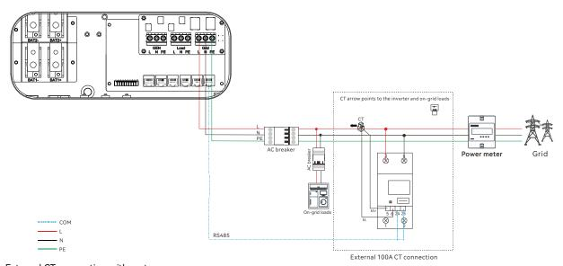
Figure 5.14. External CT connection with meter
