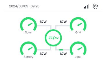
The main screen provides access to information about the inverter, solar, grid, battery, and loads. In addition, it illustrates the energy flow direction.
