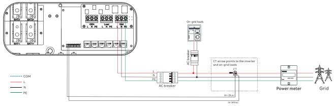
Figure 5.15. External CT connection without meter
