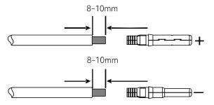
Figure 5.18. Stripping off the cable insulation
