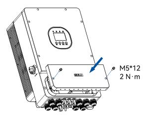
Figure 5.24. Closing the cover of the junction box
