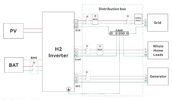
Figure 5.2. Whole home backup system connection diagram
