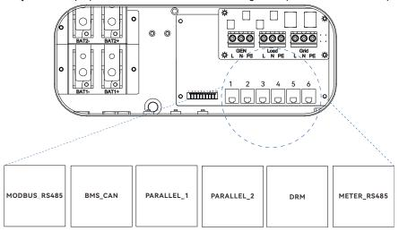
Figure 5.9. RJ45 ports
