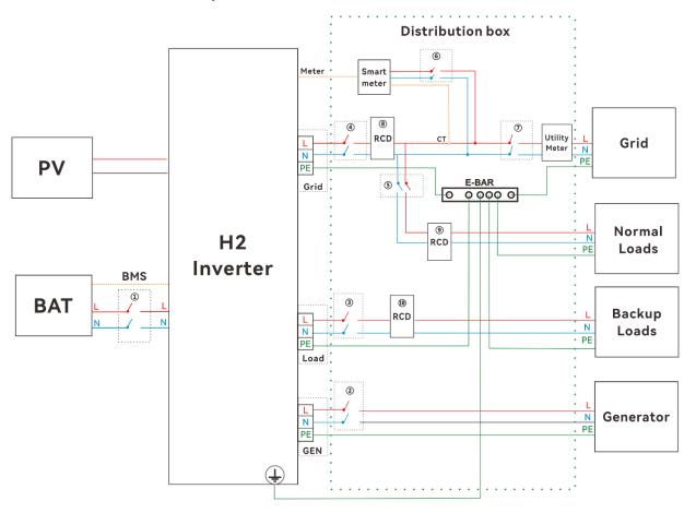
Figure 5.1. Basic system connection diagram
