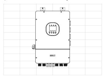
Step 3. Mount the inverter onto the mounting bracket.
