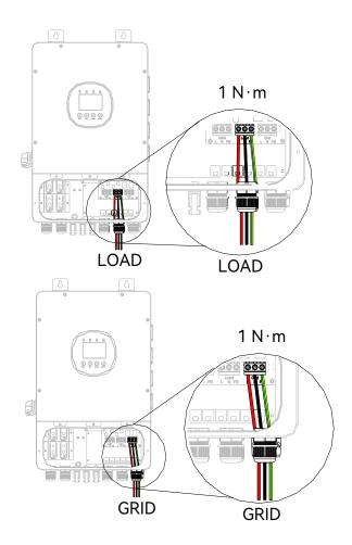
Figure 5.6. Connect the GEN, LOAD, and GRID cables
