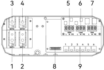
Figure 2.4 Electrical terminals in the junction box
