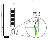
Figure 5.2. Connect the grounding cable
