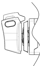
Figure 5.16. DC switch at OFF position
