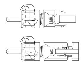
Figure 4.12 Securing the connectors
