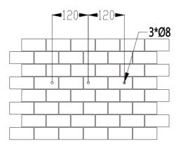
Figure 3.4 Drilling holes position
