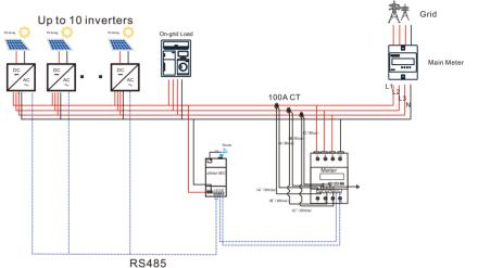
Figure 4.7 Multiple Inverter Combinations
