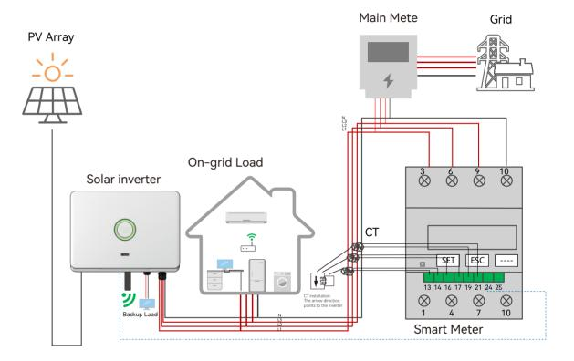
Figure 5.4 Export limit wiring schematic
