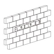
Figure 3.5 Securing the plate
