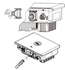
Plug in the communication module to 4G/WIFI port and secure the module by rotating the nut.
