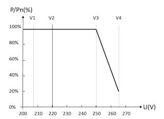
Figure 5.5 Curve for a Volt-Watt response mode (AS4777 Series)
