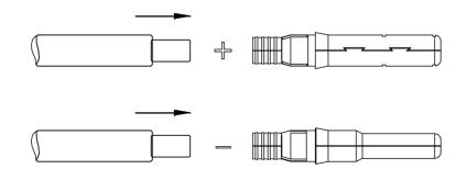
4.Insert the positive and negative cable into positive and negative connector. Gently pull the cables backward to ensure firm connection.
