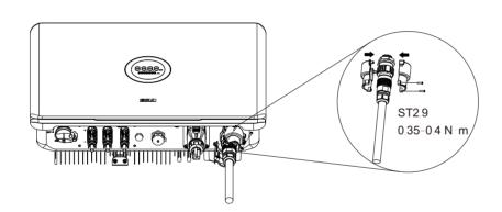
Figure 4.6 Protective covers installation
