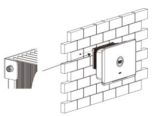
Figure 3.6 Mounting inverter
