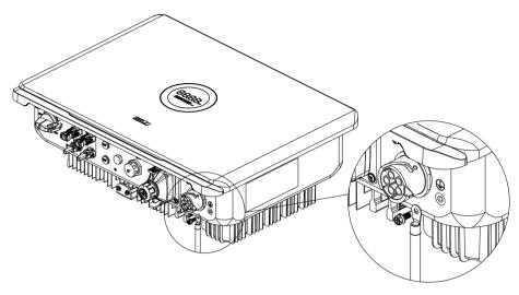
Figure 4.2 Inverter ground protection
