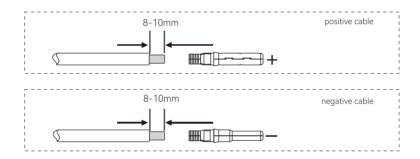
Figure 4.9 Striping off the insulation skin of cables
