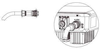
Figure 4.5 AC connector installation
