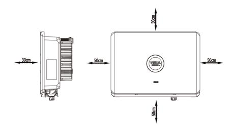
Figure 3.2 Mounting Clearance
