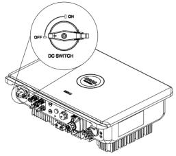
7.Connect the positive and negative connectors into positive and negative DC input terminals of the inverter, a "click" should be heard or felt when the contact cable assembly is seated correctly.
