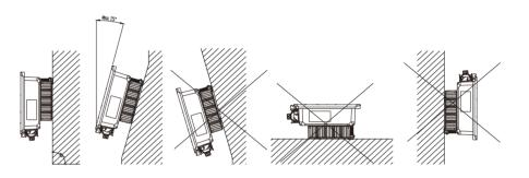
Figure 3.1 Mounting Method
