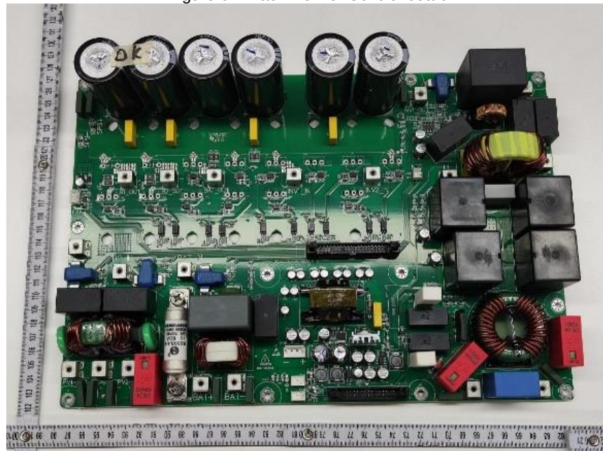
Figure 62. Front view of Main power board
