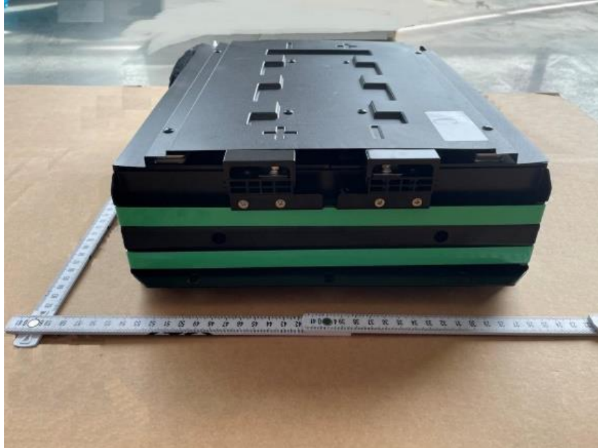
Figure 75. Battery cell side view
