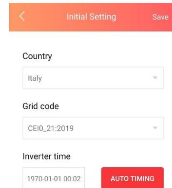
Fig 3.7 Inverter grid compliance setting
